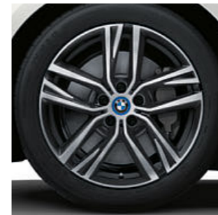
□ 18" light alloy wheels Double-spoke style 853 Bicolour Dark Grey with mixed tyres, gloss-lathed, wheel size front 8.5J x 18 with 245/45 R18 tyres, wheel size rear 9J x 18 with 255/45 R18 tyres. 1
